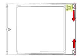
Step 4: To move the rails, use a Philips head screw driver to remove the sheet metal screw on each rail. Lift up on the rail and pull toward you to remove the rail. Find your desired mounting depth before dropping your rail into place. The sheet metal screw can be discarded. The screw is used to secure rail during shipping.
