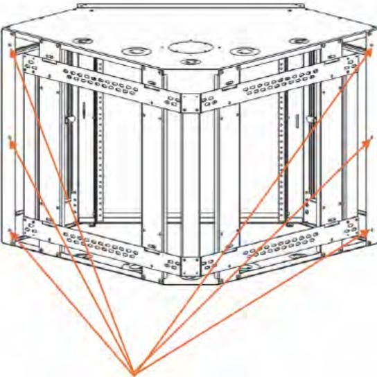
Install screws from the inside of the cabinet(not provided) in these six (6) locations BEFORE installing any equipment in the cabinet.
