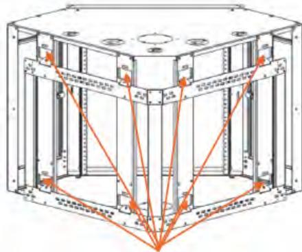
Once mounting frame is secured to corner, lift and lower the wall mount cabinet so that each of the eight (8) beveled tabs slide into the eight (8) slots in the back of the wall mount cabinet.
