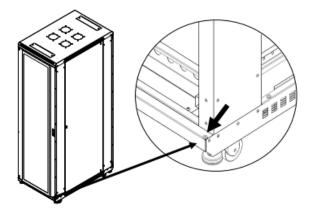
**Step 2:**Remove the cable pass thorough covers by unscrewing the Phillips head screws in the panel.
