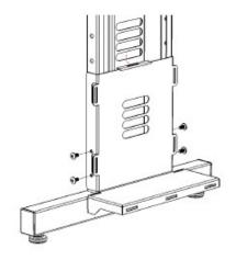
Line up holes and insert 1/4-20" screws and secure.
