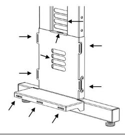
Use hook and loop strap to secure CPU or unit to CPU holder by lacing the strap through any of the 10 tie points.
