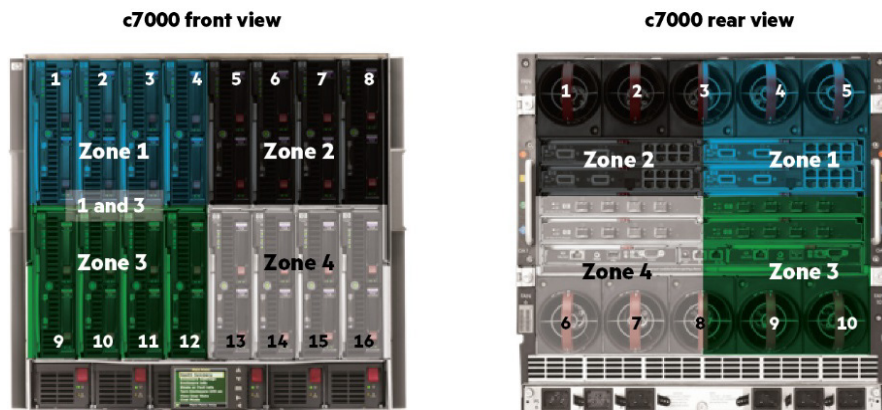
Figure 18. c7000 Enclosure divided into four cooling zones with fans in each zone
