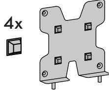
b Bump-on placement for 35-38mm pole attachment.
