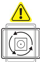
**WARNING!** Mini PC may fall out of brackets. Install the Portrait/Landscape rotation stop screw to keep monitor from rotating through the portrait/landscape rotation. Failure to follow these instructions may result in the Mini PC falling out of the brackets and could result in equipment damage and/or personal injury.
