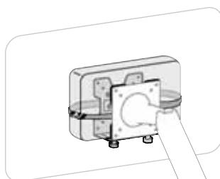
**IMPORTANT!** This product adds an additional 2 lbs. (1 kg) to your mounting solution. When mounting between a monitor and VESA plate, the mounting solution's monitor weight capacity must be reduced by 2 lbs. (1 kg) when using standard monitors and Mini PCs which when combined are less than or equal to 2.5" (64 mm) thick. Additional reduction will be required if the combined monitors and Mini PC are greater than 2.5" (64 mm) thick.
