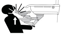
WARNING: E-Brake cover could be broken if the keyboard arm is panned and slammed into the stowed position.
