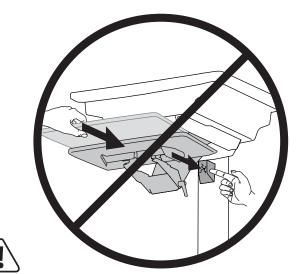
WARNING: E-Brake cover could be broken if the keyboard arm is panned and slammed into the stowed position.
