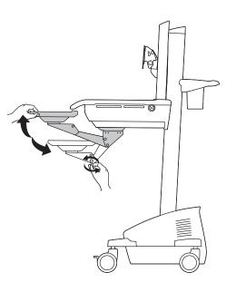
WARNING: Keyboard tray can spring up when lever is released.
