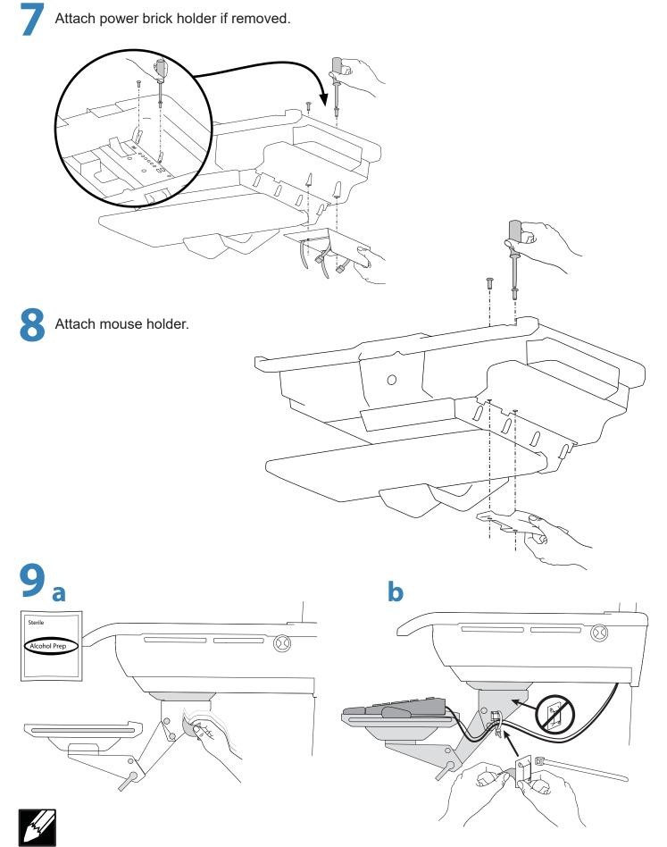
**NOTE:** Keyboard and mouse cables need to be routed as shown. Wipe location with alcohol pad before sticking the cable managment bracket to the keyboard arm
