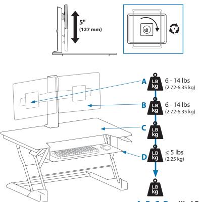
A+B+C+D ≤ WorkFit-T: 25.3 lbs (11.48 kg) WorkFit-TL: 30.3 lbs (13.74 kg) WorkFit-TLE: 30.3 lbs (13.74 kg)
