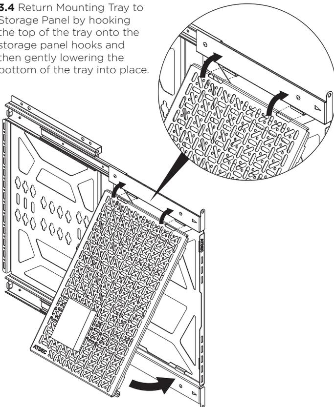
**3.5** Once the Mounting Tray is engaged, slide the Locking Tabs outward to secure the Mounting Tray in place.
