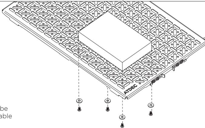
**Note:** Components can also be mounted to the Tray using cable ties or hook and loop strips.
