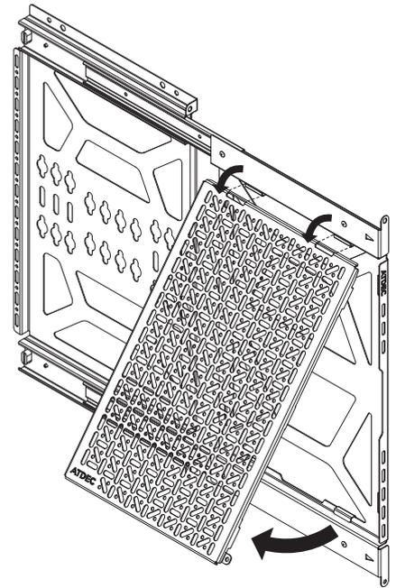
**3.3** Place media components on Mounting Tray by aligning the mounting holes of components to the hole pattern on Mounting Tray. Use the fasteners provided with the component and washers (if required) to attach the component to the Mounting Tray.
