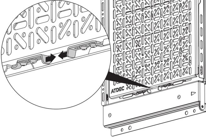
**3.2** Lift out the bottom of the tray and unhook it from the top tabs.
