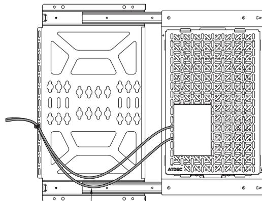
Allow slack in cable for sliding movement of tray
