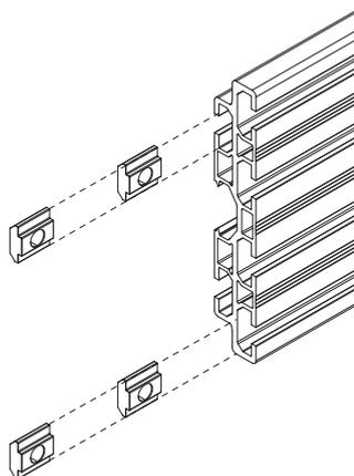
**2.4** Attach Storage Panel to rail and reassemble the end cap and screw.
