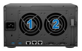
3 Remove the four screws that secure the fan panel.
