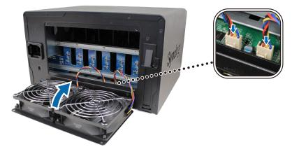
**6** Replace and tighten the four screws removed in step 3.
