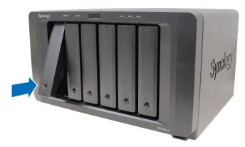
2 Pull out the hard drive tray handle as shown below to remove the hard drive tray.
