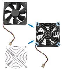
**b** Attach the fan case (with the fan cable within the fan pointing at the bottom-right corner) to the new fan, then tighten the screws to secure the fan case.
