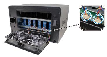
$\boldsymbol{c}\$  Remove the screws that secure the fan from the fan case.
