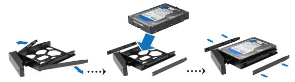
• For 2.5" drives: Remove the fastening panels from the sides of the drive tray and store them in a safe place. Place the drive in the area of the drive tray indicated by a blue rectangle below. Turn the tray upside down and tighten the screws to secure the drive in place.
