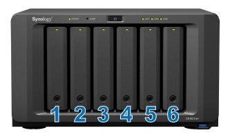
**Note:** If you plan to create a RAID volume, we recommend installing drives of identical size to make the best use of drive capacity.
