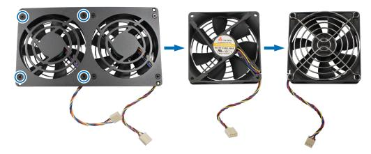
**d** Remove the screws that secure the fan guard from the malfunctioning fan.
