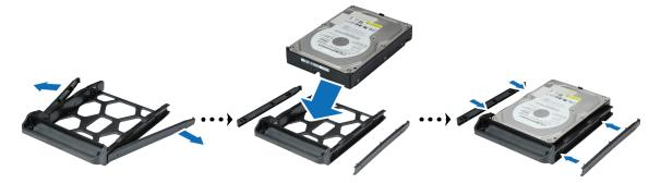
• For 2.5" drives: Remove the fastening panels from the sides of the drive tray and put them in a safe place. Place the drive in the blue area (shown below) of the drive tray, turn the tray upside down, and then tighten the screws provided to secure the drive.
