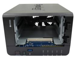
**Note:** When you remove the drive trays, sensitive internal components are exposed. Avoid touching anything other than the memory assembly when removing or adding memory.
