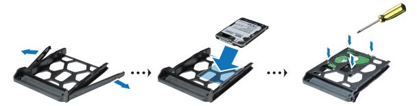
4 Insert the loaded drive tray into the empty drive bay. Make sure the side marked **"UP**" is facing up, and insert the drive tray into the empty drive bay. You should hear a click when the tray is locked in place.
