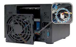
c Remove the screws that secure the fan guard and fan case from the malfunctioning fan.
