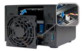
**5** Replace and tighten the four screws removed in step 2.
