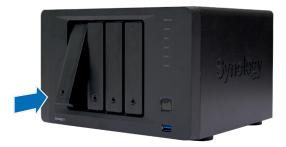
2 Pull out the hard drive tray handle as shown below to remove the hard drive tray.
