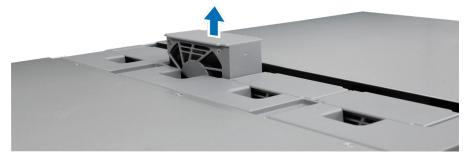
5 Prepare a new fan, and slide it into the RackStation. Make sure the fan is aligned properly as illustrated below.
