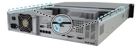
**b** Put back and fasten the screw you removed in step 2-a.
