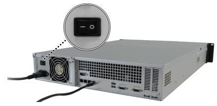
4 Press the power button to turn on the RackStation.
