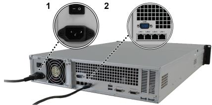
3 Make sure the Power Supply On/Off Switch is turned on ("|").
