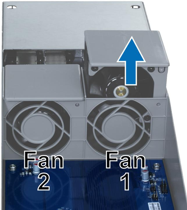
**2** Prepare a new fan, align the arrow to point at the back panel as illustrated below, and insert it back into the fan slot.
