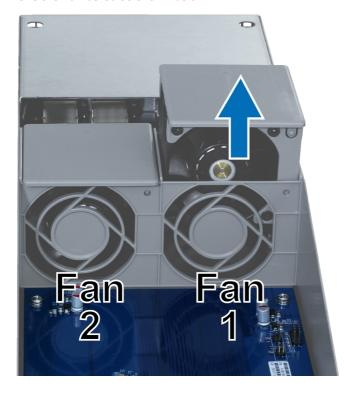
**2** Prepare a new fan, align the arrow to point at the back panel as illustrated below, and insert it into the empty slot.
