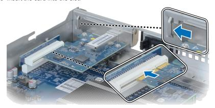
**d** Push back the tab to secure the newly inserted card.
