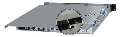
**b** Fasten the two screws you loosened in step 2-a.
