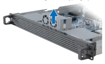
**4** Prepare a new fan mudule and insert it into the empty slot using the orientation illustrated below.
