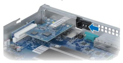
**Note:** Make sure the connector is fully inserted. Otherwise, the network interface card might not be able to function properly.
